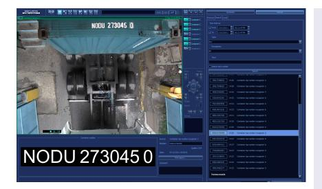
SecurOS CARGO is an intelligent video analytics module for the SecurOS video management platform providing recognition of cargo container ISO codes in a variety of applications. It implements the most advanced native image processing software, the ISS SecurOS framework, and advanced algorithms for the recognition of codes on cargo containers.
