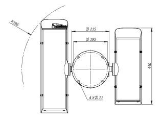
The unit cannot be installed upside-down nor horizontally
